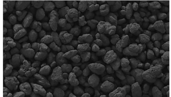
Katalox Light® is an advanced catalytic filter material used for filtering out dirt, sediments, suspended solids (down to 3 micron) and to remove Iron, Manganese, Hydrogen sulfide, Arsenic, Fluoride, Zinc, Copper, Lead other Heavy metals and radionuclide like Uranium, Radium from drinking water, process water and irrigation water.
